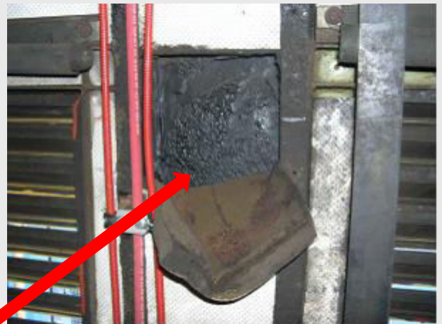
Wall coating (bitumen coating to main steel walls of train)
