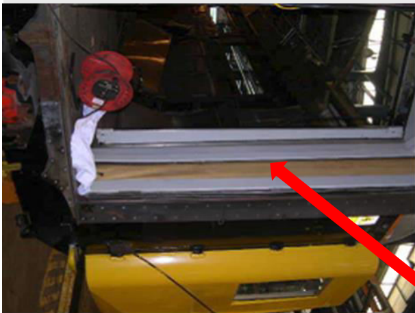
Door surround panel (panels around carriage end doors & wall board/panel)
