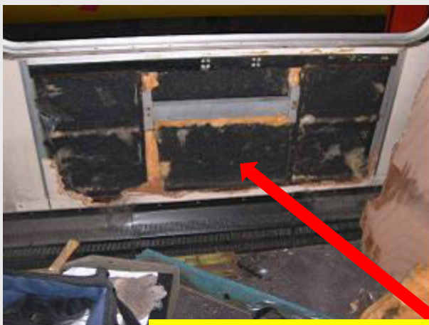
Wall coating (bitumen coating to main steel walls of train)
