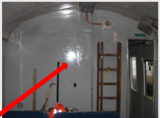
Door surround panel (panels around carriage end doors & wall board/panel)
